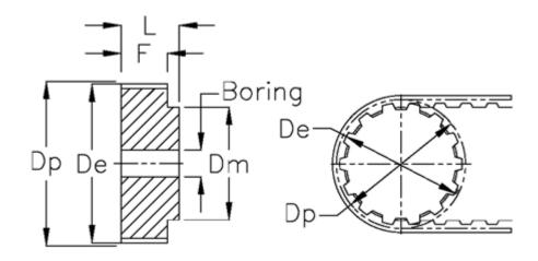
Type = T5Belt width = - 10 mm Weight = 0.2= 69.2 De Dm = 45 Dp = 70.2 F = 15 = 21 L Pre-drilled = 8 Tooth number = 44
